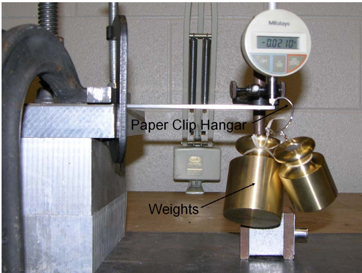
Figure 8. Cantilevered Beam with Weights Applied
